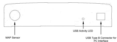
Below is the right hand side of the MAPECU3 showing connector and LED indicator layout:
