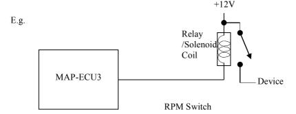
**Note**: The MAPECU3 already contains a diode connected to each Switched Output and +12V to suppress Back-EMF from the solenoid.
