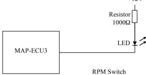
Example of shift light based on a 12V (integrated resistor) high intensity Light Emitting Diode (LED):
