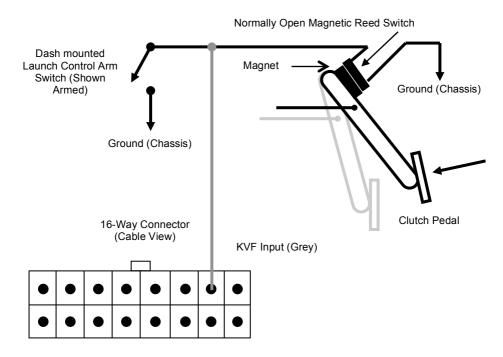
**Note**: A micro switch can be used instead of a Normally Open (NO) magnetic reed switch. Connect the common of the micro switch to Ground and the Normally Open (NO) connection to the LC Input. The micro switch should be closed when your foot is off the clutch pedal.
