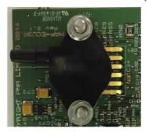
WARNING! DO NOT ATTEMPT TO REMOVE THE VACUUM HOSE BY BENDING IT SIDEWAYS OTHERWISE YOU MAY BREAK THE NIPPLE OFF THE SENSOR. PULL THE VACUUM HOSE OFF STRAIGHT OR CUT OFF THE SLICE OF VACUUM HOSE THAT SECURES THE REMAINING HOSE.
