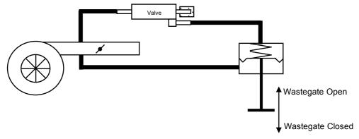
In External mode, **more** duty cycle bleeds more boost pressure from the wastegate canister, therefore **reduces** boost.
