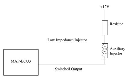
**Note:** Low impedance injectors **must** be **Saturation** types designed for a series resistor, **not** Peak-hold low impedance injectors.
