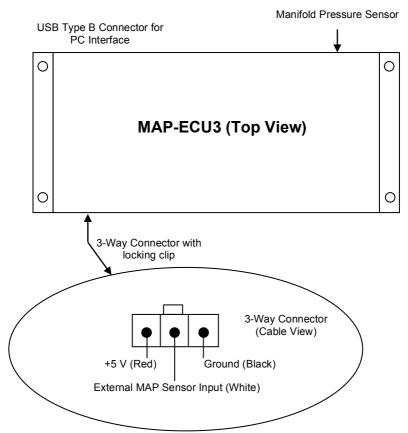
Various External MAP Sensors can be connected to the MAPECU3, e.g. GM 2-Bar, GM 3-Bar, AEM 5-Bar. Configuration is completed using MAPCAL3. An external MAP sensor must be a linear 5 Volt type where minimum voltage equals vacuum and maximum voltage is maximum boost. The wiring is as follows:
