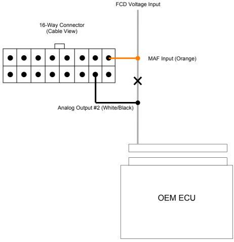
**Note**: If the MAPECU3 is providing the MAF, MAP or KVF signal from it's fuel table, an additional FCD function is not required as the fuel table can clamp the signal. See **Fuel Cut Defeat using the fuel table** elsewhere in this manual.
