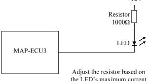
Example of LBR indicator based on a 12V (integrated resistor) high intensity Light Emitting Diode (LED) or light bulb:
