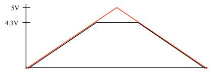
Red Line = Input Voltage Black Line = Output Voltage
